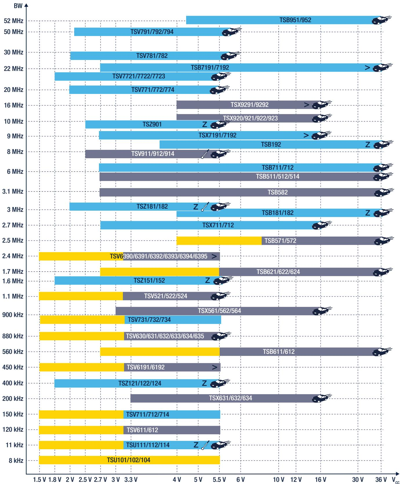
Legend: High precision (blue), General purpose (grey), Low power (yellow), Automotive (car icon), Z Zero-drift, > Uncompensated, H High temperature (thermometer icon)
