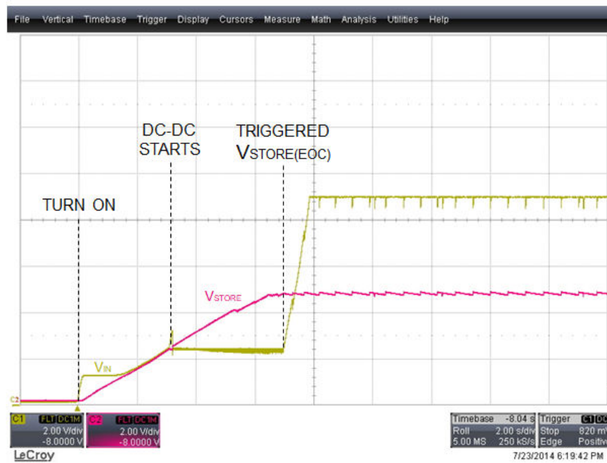
Figure 14. Buck-boost start-up ( I_{IN} = 5 \mu A )
