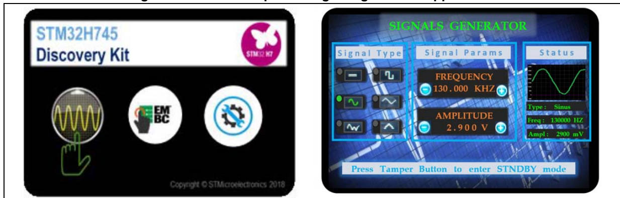
Figure 71. Oscilloscope and signals generator application
