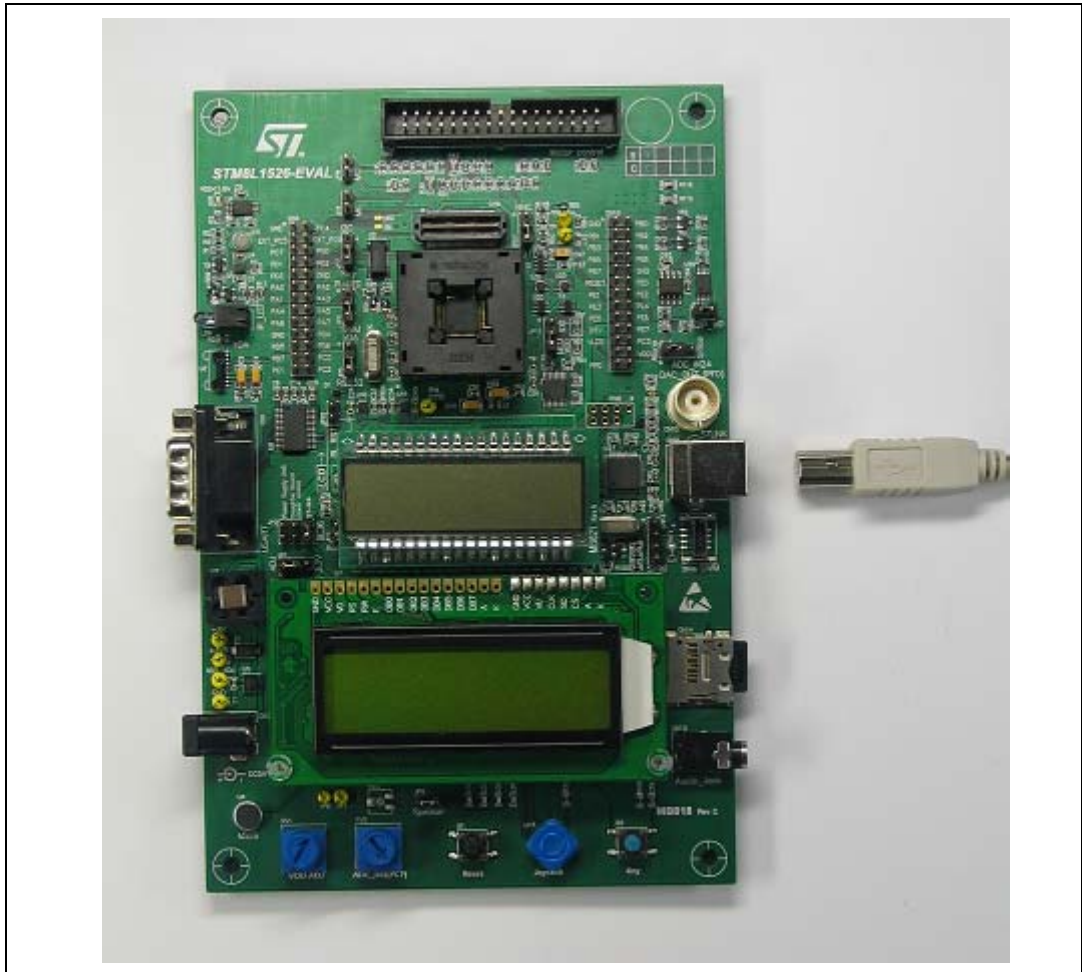
Figure 23. Connecting the debug instrument to the STM8L152x-EVAL evaluation board
