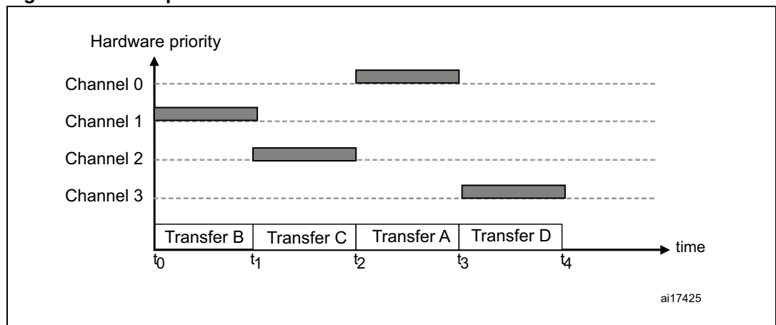
Figure 10. Example case 3: DMA channel data transfers as a function of time
