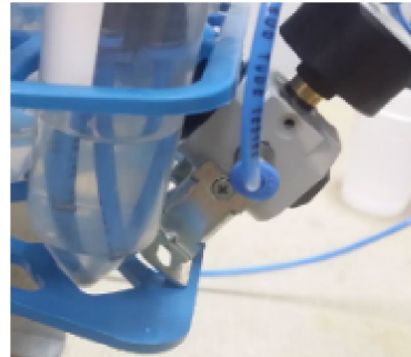
Figure 17. LPS27HHW immersed in water for air overpressure
