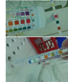
Figure 16. Chlorine, bromine, saltwater and detergent tests
