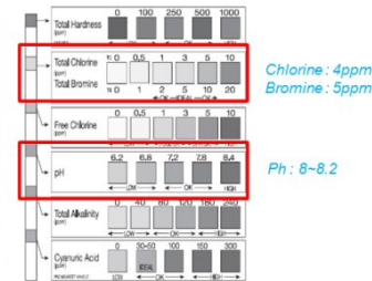
Figure 16. Chlorine, bromine, saltwater and detergent tests
