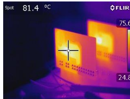
Without heatsink @ Pin = 200W
