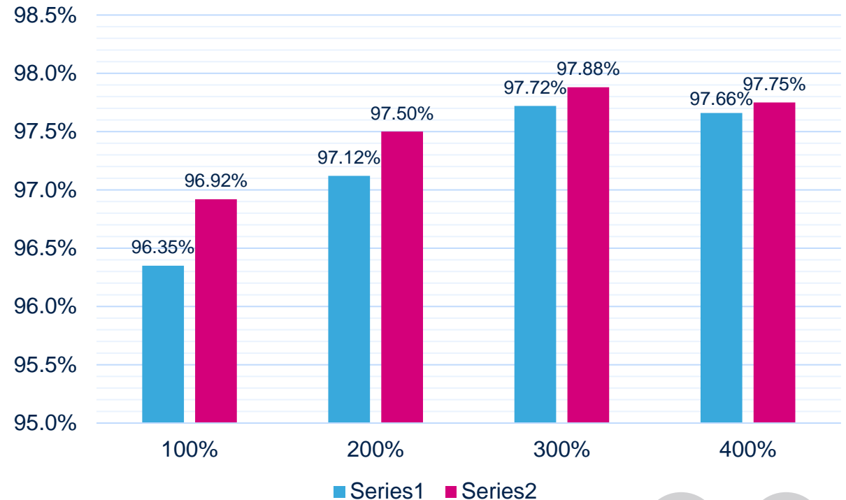
Efficiency of 1 kW PFC vs. output power load
