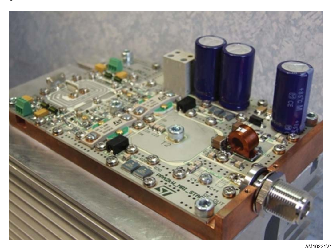
Figure 4. 2 kW MRI final assembled board
