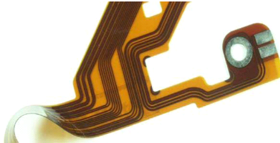
Figure 5. Flexible PCB (FPC)
