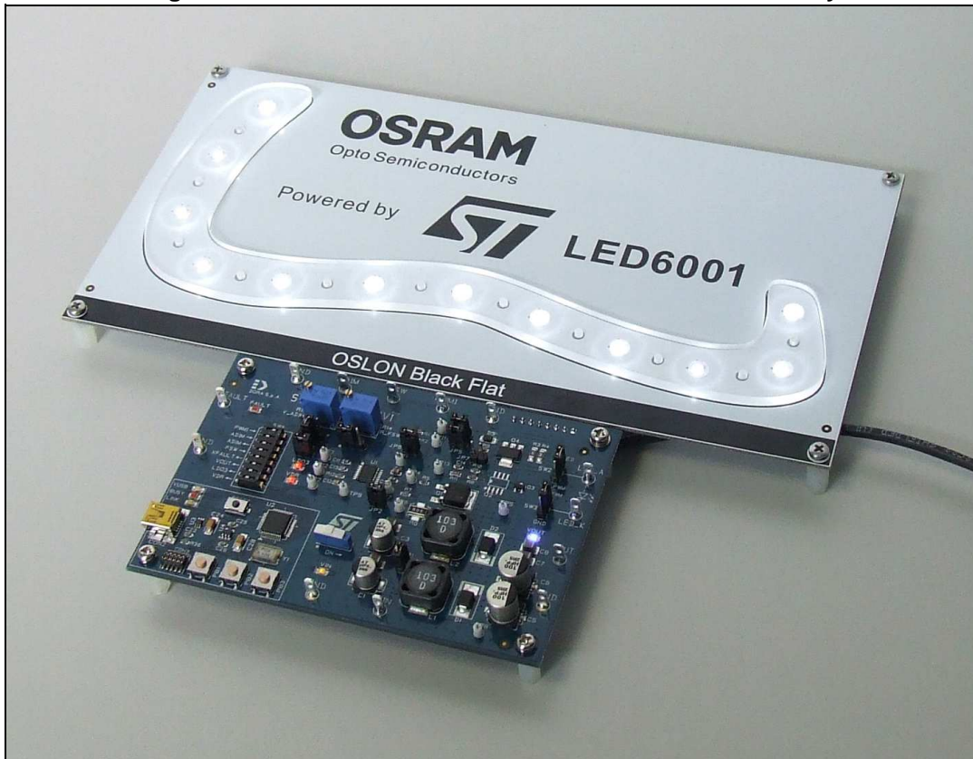
Figure 16. OSLON_DTRL_L and STEVAL-ILL048V1 assembly
