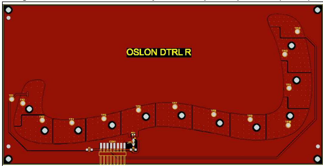
Figure 19. OSLON_DTRL_R board layout and components placement (bottom)
