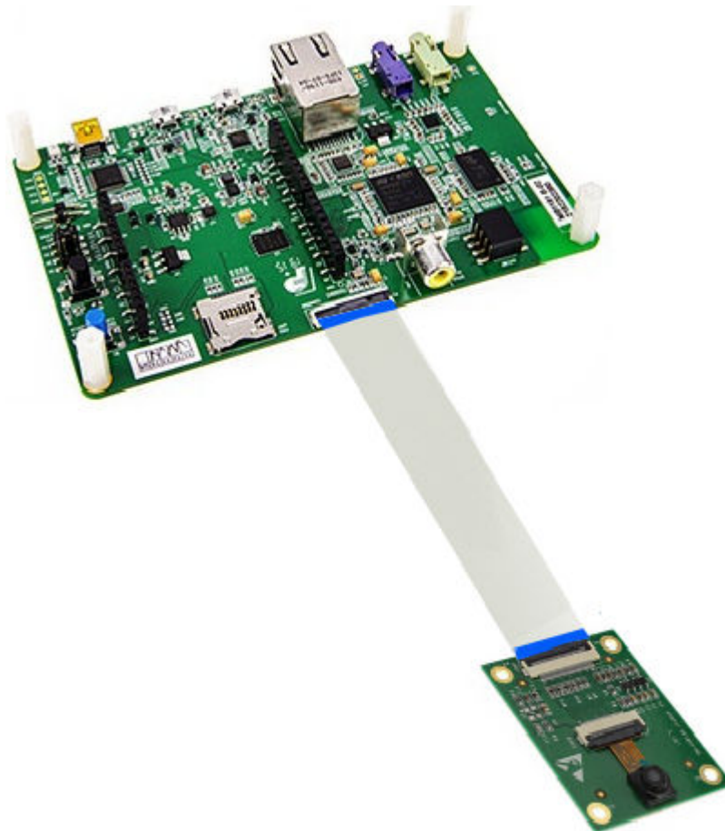
Figure 50. 32F746GDISCOVERY and STM32F4DIS-CAM interconnection
