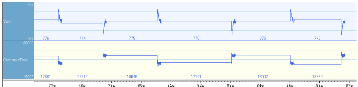
Figure 94. Timeline view with an adjusted scale showing the voltage transients and change in the duty cycle
