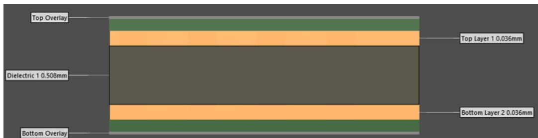
Figure 1. Two layers application board stack-up
