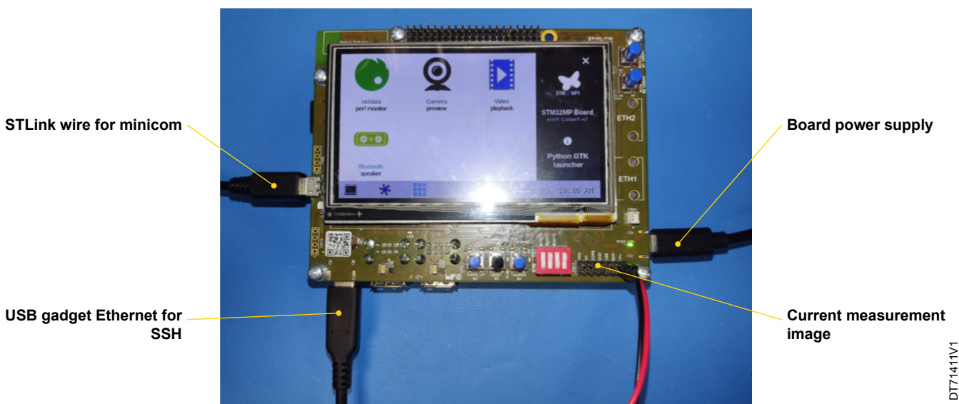
Figure 1. Board with cables
