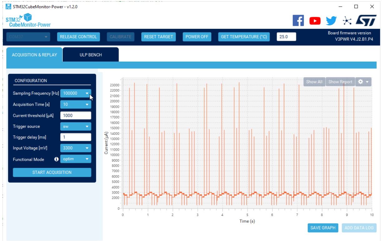
Figure 13. STLINK-V3PWR configuration and start acquisition with STM32CubeMonitor-Power
