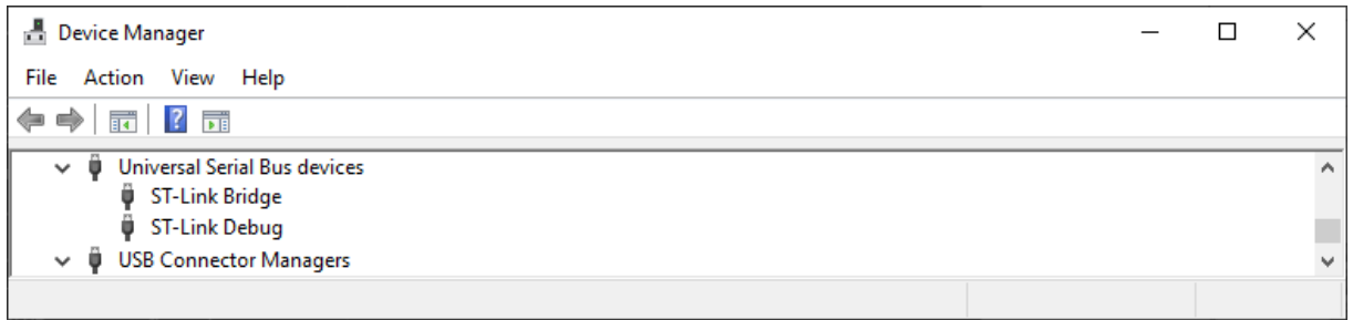
Figure 8. STLINK-V3PWR bridge USB device in a Windows 10 environment
