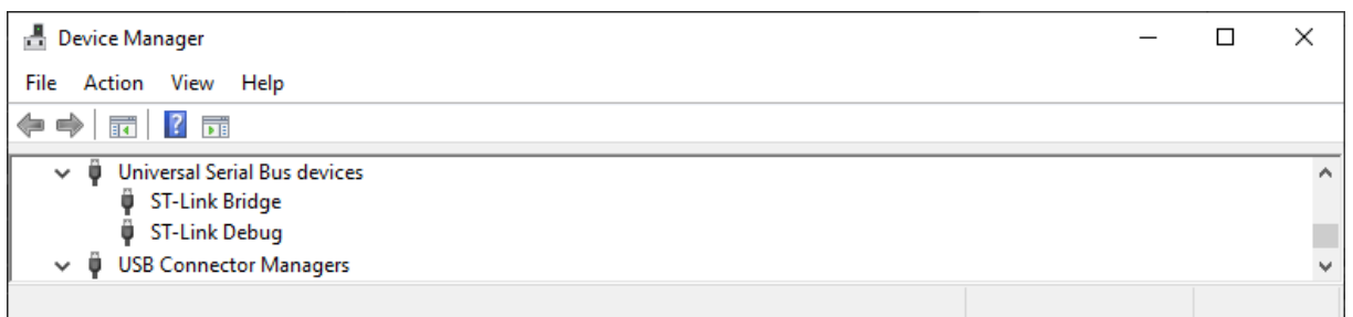
Figure 6. STLINK-V3PWR debug USB device in a Windows 10 environment
