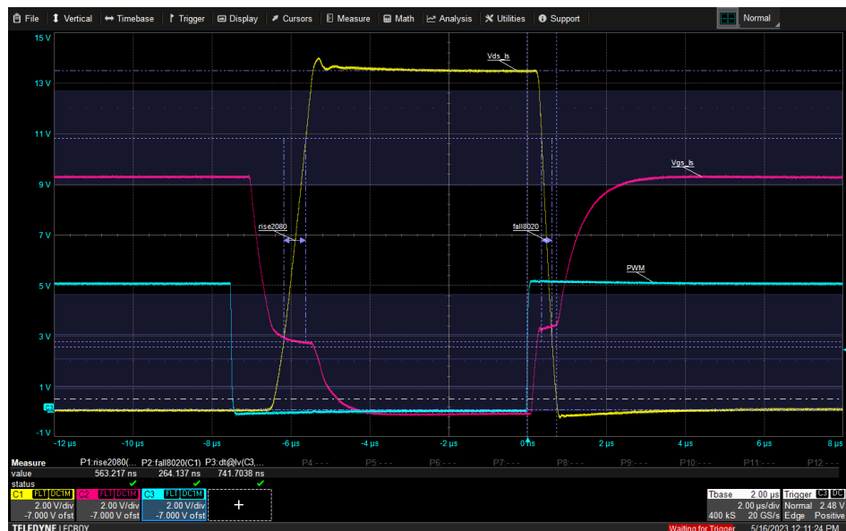
Figure 9. Measured switching waveforms with asymmetrical gate driving
