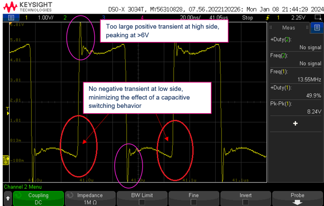
Figure 39. RFO transients showing inductive switching behavior
