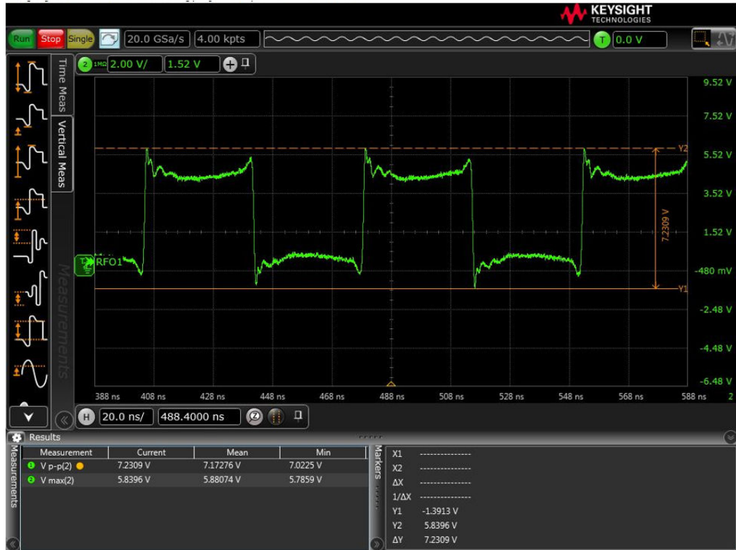
Figure 38. RFO signal with capacitive transient behavior
