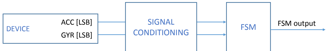
Figure 2. State machine in the ASM330LHBG1
