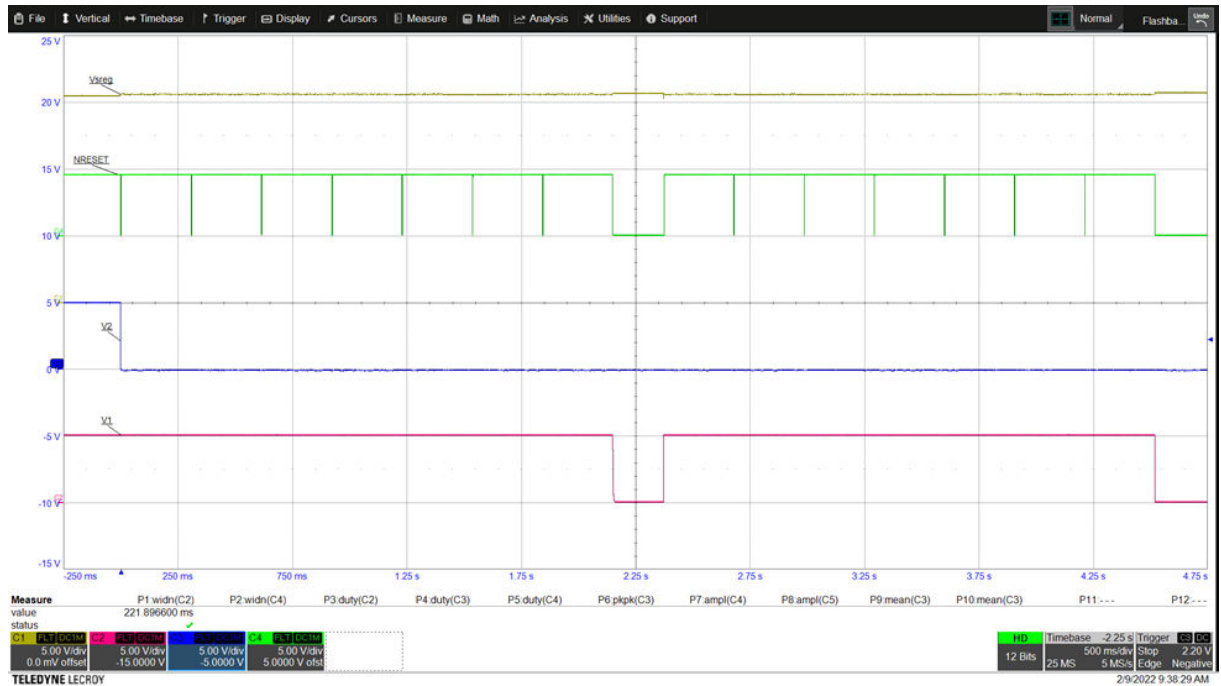
Figure 16. Oscilloscope consecutive watchdog failures
