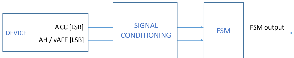
Figure 2. State machine in the ST1VAFE3BX
