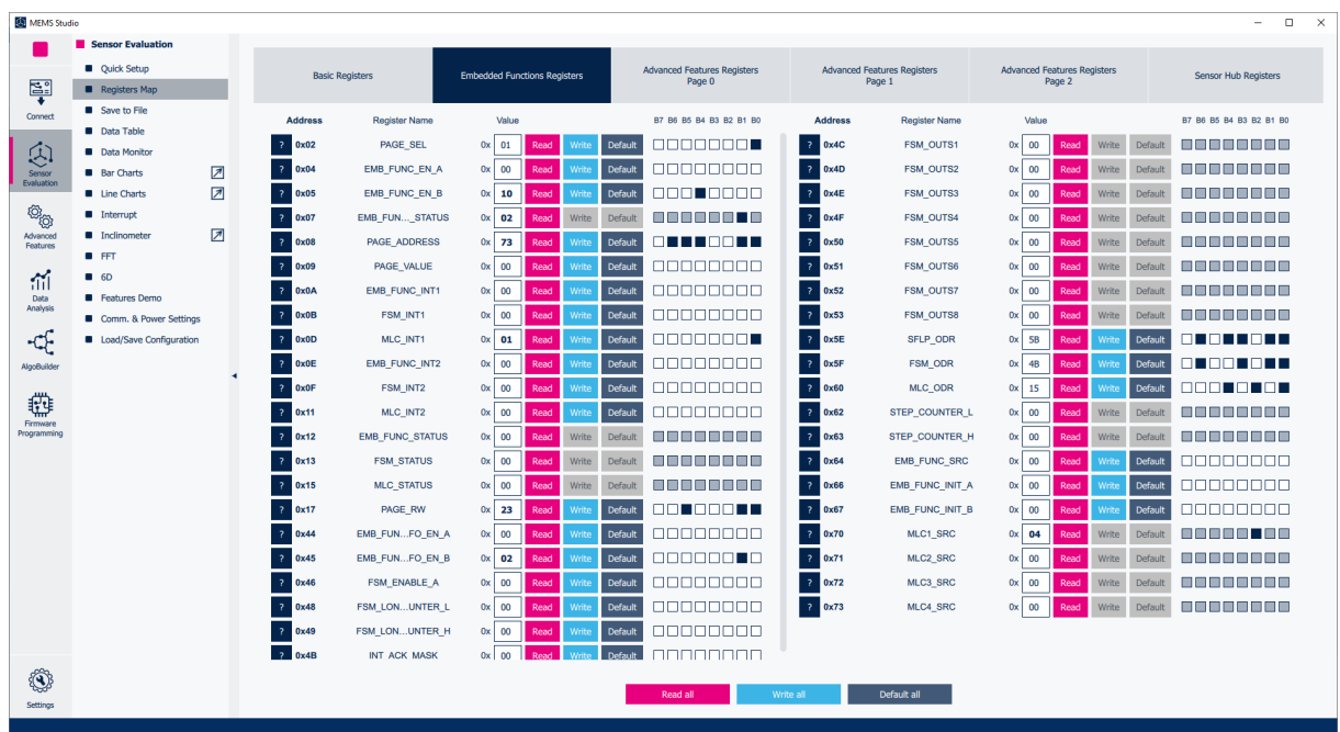
Figure 38. MEMS Studio - machine learning core source registers
