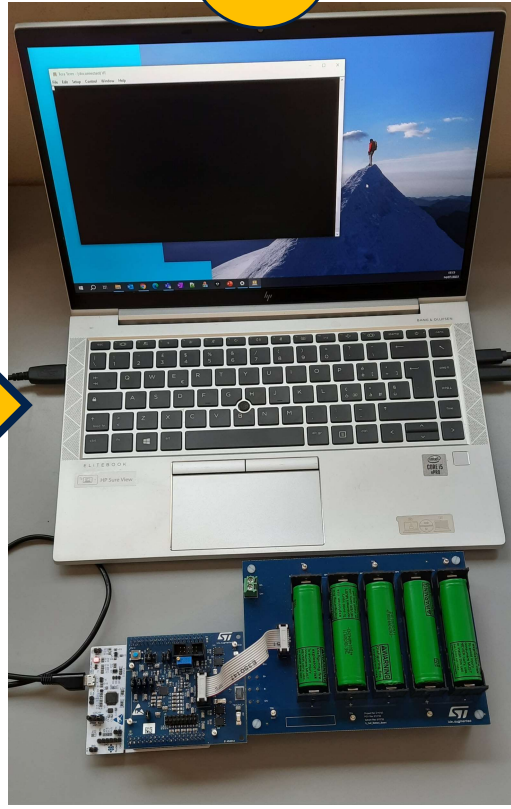
Open the terminal on the laptop and select the corresponding serial port (and set COM speed @ 115200)
