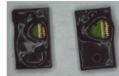
Example of de-soldering at 350°C
