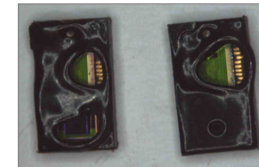
Example of de-soldering at 350°C
