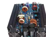
STEVAL-ISA172V2 2 kW fully digital AC-DC power supply (D-SMPS)
