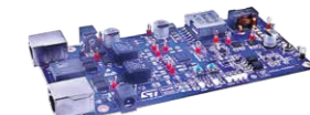
STEVAL-POE006V1 3.3 V/20 A, active clamp forward converter, power over Ethernet (PoE) IEEE 802.3bt compliant reference design
