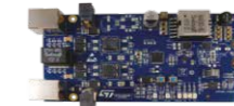
STEVAL-POE002V1 5 V/8 A, synchronous flyback converter, power over Ethernet (PoE) IEEE 802.3bt compliant reference design
