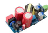
EVLVIPGAN50FL 15 V - 50 W QR SSR flyback with HV GaN converter and synchronous rectification
