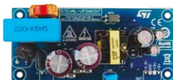
STEVAL-VP26K01F Three outputs, isolated SSR flyback converter with extended input voltage range for Smart meter and power Line communication
