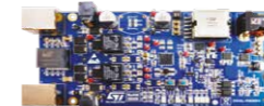
STEVAL-POE005V1 12 V/8 A, active clamp forward converter, power over Ethernet (PoE) IEEE 802.3bt compliant reference design
