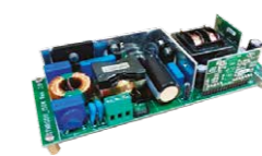
EVLSTNRG011-150 EVL011A150ADP 12 V - 150 W power supply based on TM PFC and HB LLC digital combo controller
