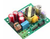
EVLONE65W 65 W USB Type-C power delivery reference design with integrated GaN
