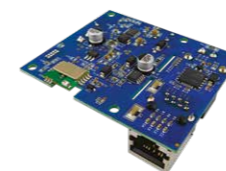
STEVAL-POEL45W1 45 W PoE powered LED lighting with BLE control
