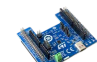
X-NUCLEO-SRC1M1 USB Type-C power delivery source expansion board based on TCPP02-M18
