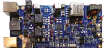
STEVAL-POE003V1 5 V/20 A, active clamp forward converter, power over Ethernet (PoE) - IEEE 802.3bt compliant reference design
