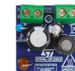
STEVAL-VP12201B 15 V/200 mA buck converter
