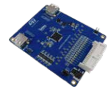
AEK-POW-BMS63EN Battery management system module
