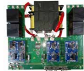
STDES-DABBIDIR 25 kW dual active Bridge (DAB) bidirectional power converter for EV charging and BESS
