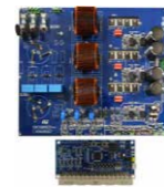
STDES-VRECTFD 15 kW, three-level, three-phase Vienna rectifier with digital control for power factor correction
