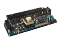
STEVAL-DPSLLCK1 3 kW Full Bridge LLC resonant digital power supply
