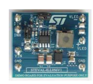
STEVAL-ILL056V1 3 A Buck LED driver board based on the LED5000
