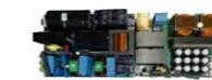
STDES-3KWTLCP 3 kW telecom rectifier reference design with Totem-Pole PFC and LLC converter
