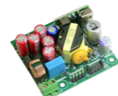
EVLONEMP Very high density board- 65 W multi-port (USB Type-C and USB Type-A) power delivery with integrated GaN
