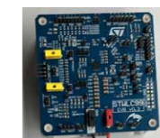
STEVAL-WLC99RX1 Qi-compatible wireless power receiver for 70 W applications
