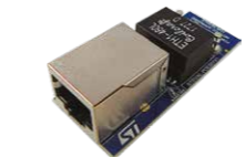
STEVAL-POE001V1 Power over Ethernet (PoE) - IEEE 802.3bt compliant interface
