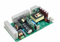
EVL400W-80PL 12 V - 400 W adapter based on CCM PFC and HB LLC analog controller
