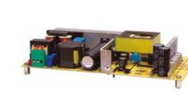
EVLCMB1-AIO210W 12 V - 210 W adapter based on TM PFC and HB LLC analog combo controller
