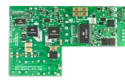
EVLONE140W 140 W USB-PD 3.1 EPR certified reference design with integrated controller and GaN
