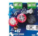
STEVAL-VP319X1B 5 V/600 mA buck converter
