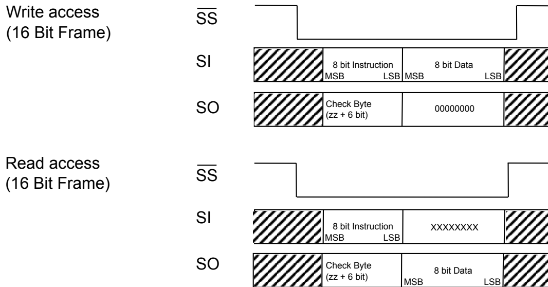
Figure 29. Standard SPI frame
