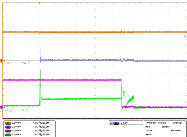
Figure 44. Output short-circuit during operation 5 V channel (Differential thermal protection)
