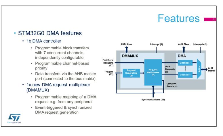
Two units are in charge of handling DMA transfers: the DMA request multiplexer (DMAMUX) and the DMA controller.
