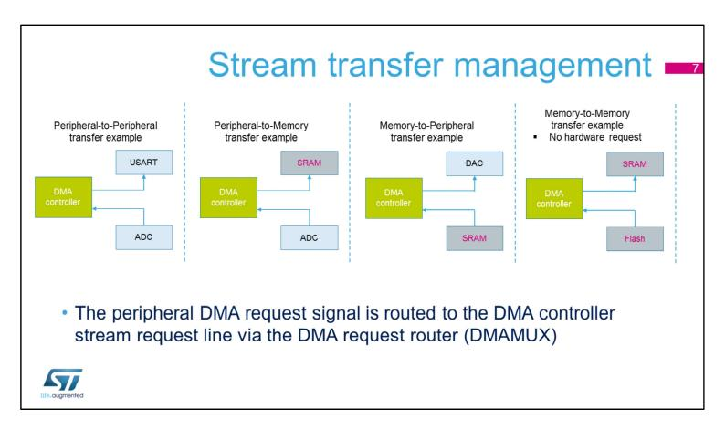
Memory-to-memory mode allows transfers from one address location to another without a hardware request. Once the stream is configured and enabled, the transfer starts immediately. When data is transferred to or from a peripheral, the hardware request coming from the selected peripheral is used to trigger the data transfer on the DMA Peripheral port. Once the transfer is completed, the request is acknowledged.
