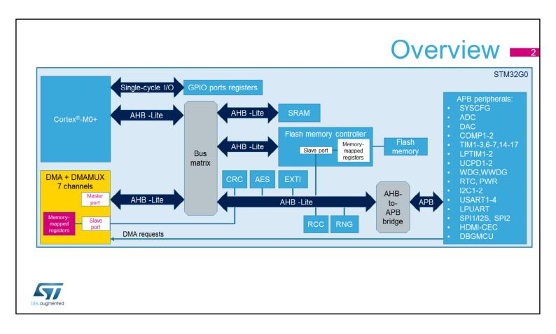
The Direct memory access (DMA) embedded in the STM32G0 microcontrollers is used to provide high-speed data transfers between peripherals and memory and between memory and memory. Data can be quickly moved by the DMA without any CPU action. This keeps CPU resources free for other operations The DMA channels can access any memory-mapped location, including:
