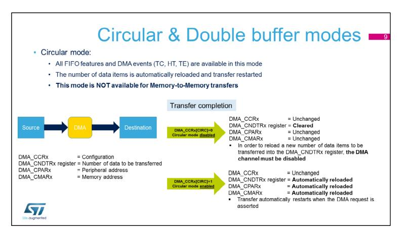
DMA controllers support Circular mode allowing to configure the number of data items to transfer once, and automatically restart the transfer after a Transfer Complete event.
