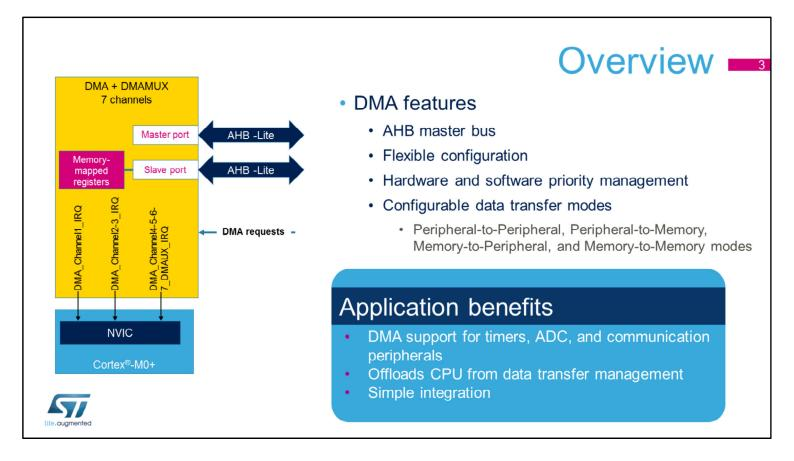
The DMA controller supports two AHB-Lite ports, one is the master port used by the DMA channels to autonomously access memory-mapped locations, memory or peripherals registers, the other is a slave port providing access to the DMA controller control and status registers.
