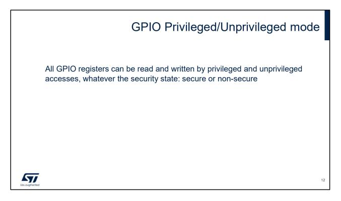
The GPIO module filters out accesses to its memorymapped registers according to the security level, but not the privilege level.
