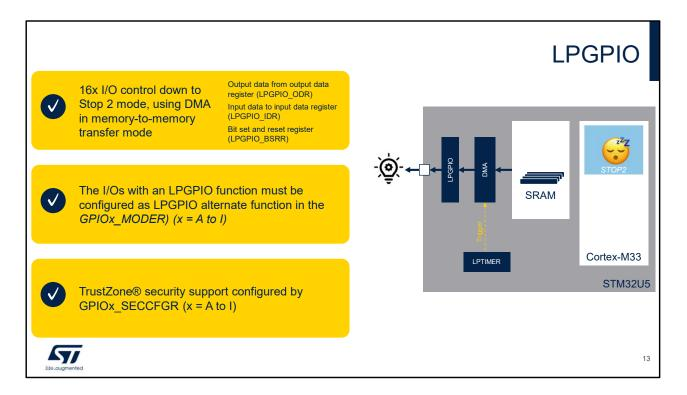
The STM32U5 supports low-power background autonomous mode (LPBAM), which allows peripherals to be functional and autonomous in Stop 0, Stop 1 and Stop 2 modes, without any software running.
