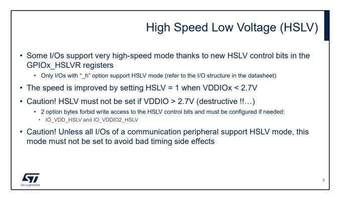
Some I/Os have the capability to increase their maximum speed at low voltage when configured in HSLV mode. They are identified by the suffix h in the data sheet.
