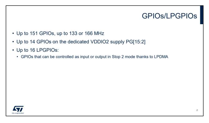
The number of GPIOs depends on the STM32U5 product and package. Refer to the product datasheet for availability of peripherals according to package size. The maximum frequency for very high-speed capable GPIOs is 166 MHz. It is 133 MHz for the other GPIOs. VDDIO2 is the external power supply for 14 I/Os: port G[15 down to 2].
