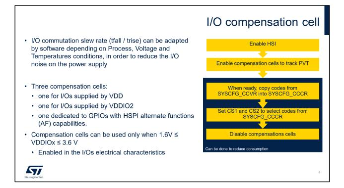
The I/O commutation slew rate, affecting rise and fall times, can be adapted by software depending on Process, Voltage and Temperatures conditions, in order to reduce the I/O noise on the power supply.
