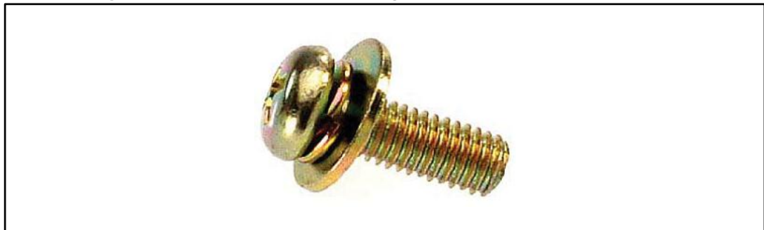
Figure 5: SEMS screw (size M3, spring washer 5.0 Φ, plain washer 7.5 Φ)
