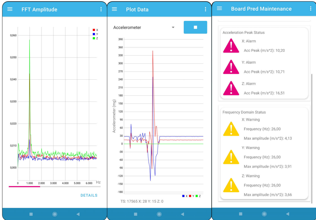
Figure 14. STBLESensor app: FFT, accelerometer data, and PdM measurements
