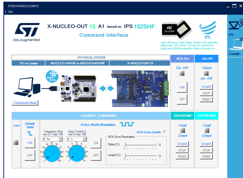
Figure 132. STSW-IFAPGUI main control panel
