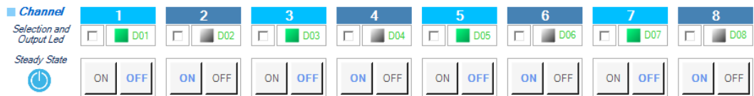
Figure 182. STSW-IFAPGUI channels 1, 3, 5, 7 Steady State ON
