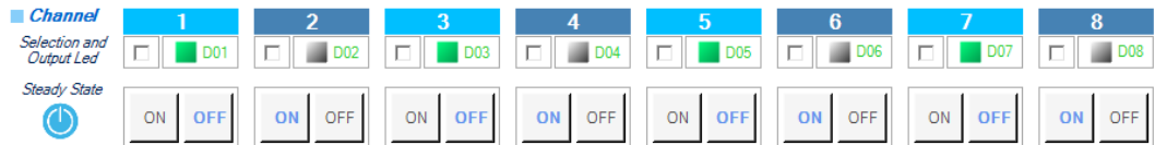
Figure 154. STSW-IFAGUI channels 1, 3, 5, 7 Steady State ON
