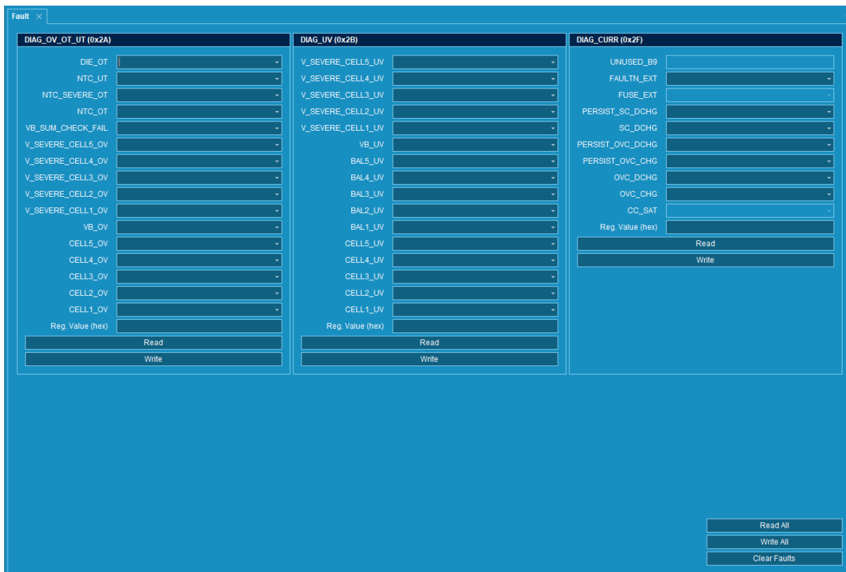
Figure 64. Fault tab display
