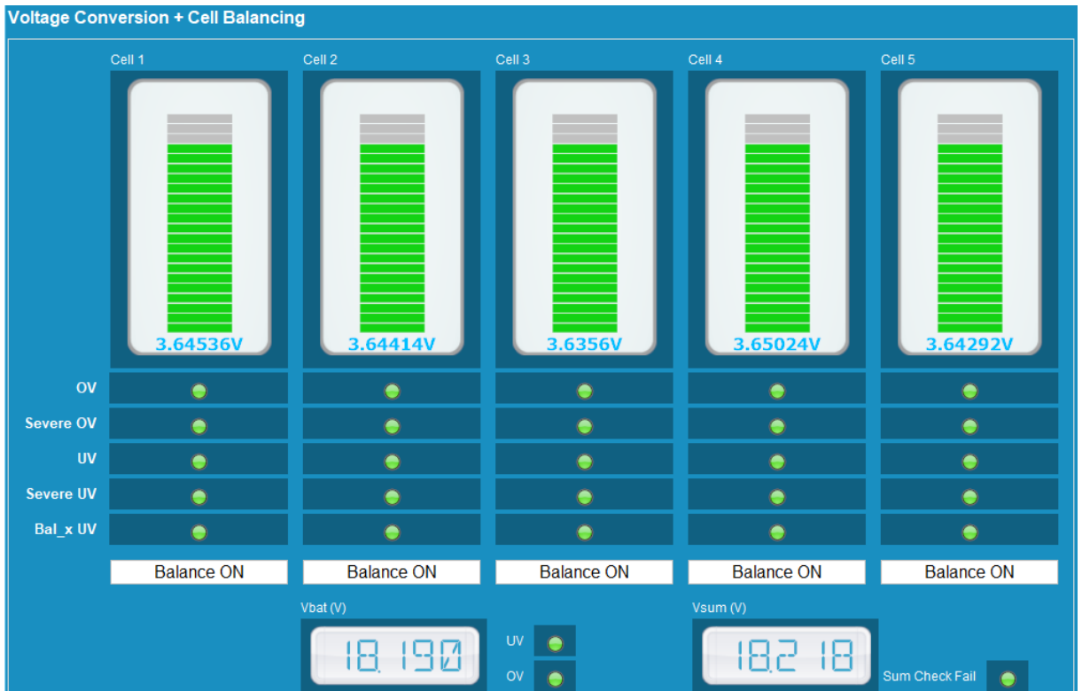
Figure 24. Voltage Conversion and Cell Balancing section
