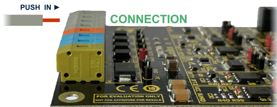
Figure 8. CN1 conductor connection
