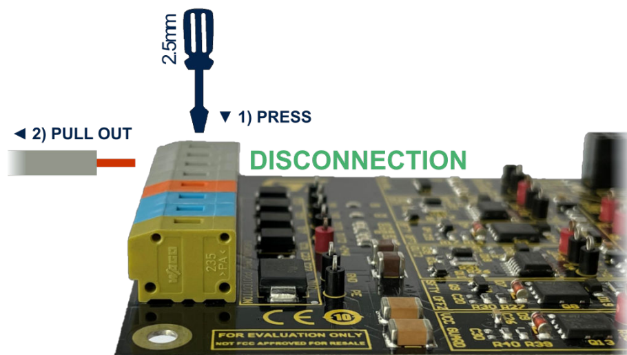
Figure 9. CN1 conductor connection
