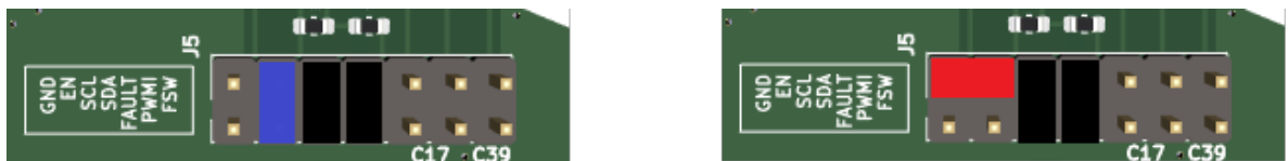
Figure 21. EN pin connection: to MCU or manually to GND
