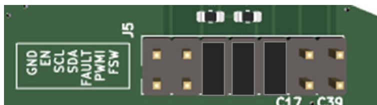
Figure 14. FAULT jumper closed on J5
