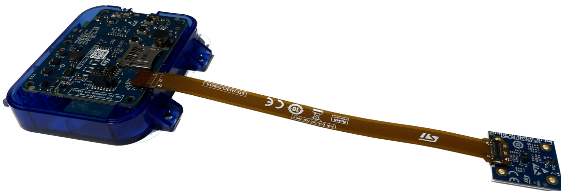
Figure 3. Plugging the flex cable onto the STWIN.box
