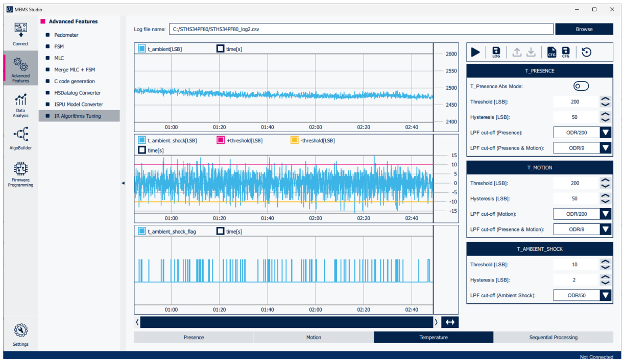
Figure 71. Ambient temperature shock detection
