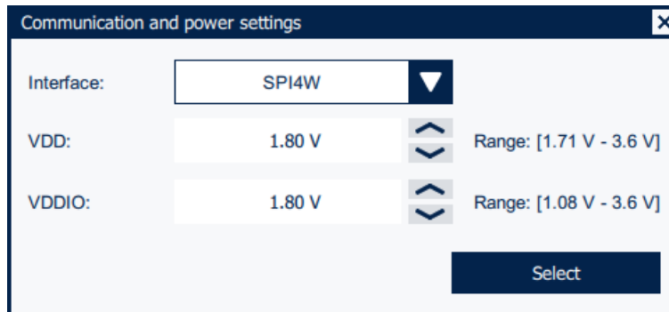
Figure 9. Advanced connection parameters
