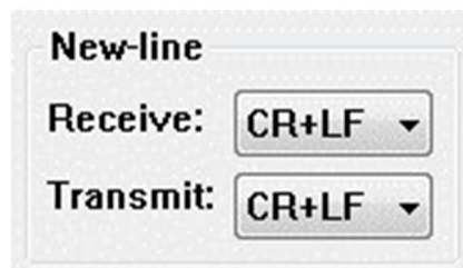
Figure 3. Example of serial COM port terminal configuration
