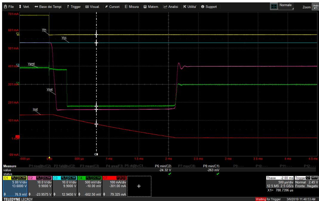
Figure 6. Measurement example ( T_{\text{DEMAG}} > t_{\text{D\_STBY}} ) with 4.7 kW GND resistor
