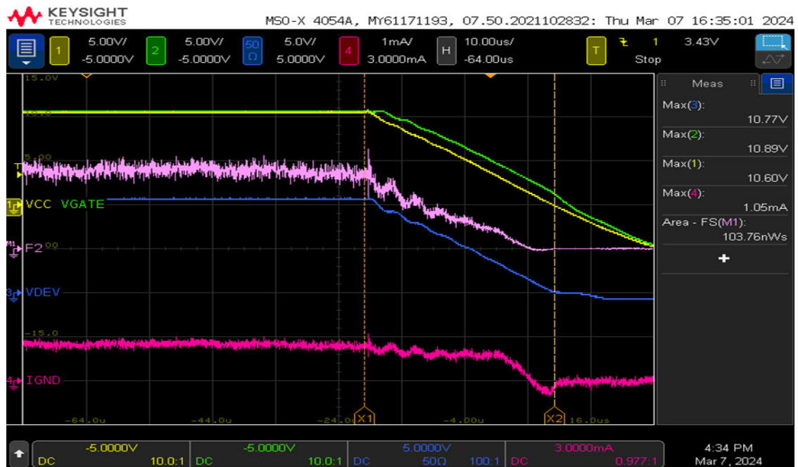
Figure 8. Reverse battery test VNQ9080AJ
