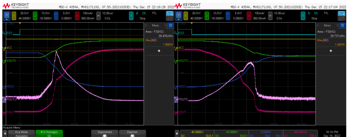
Figure 36. Slew rate and switching losses (VNQ9080AJ, VW passat B6 –tail & brake)
