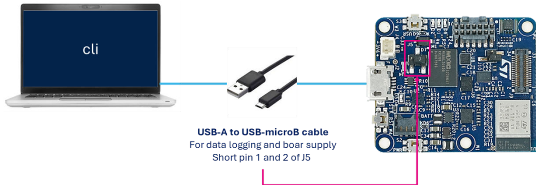
Figure 37. How to connect STEVAL-PROTEUS to a PC for USB WCID data logging
