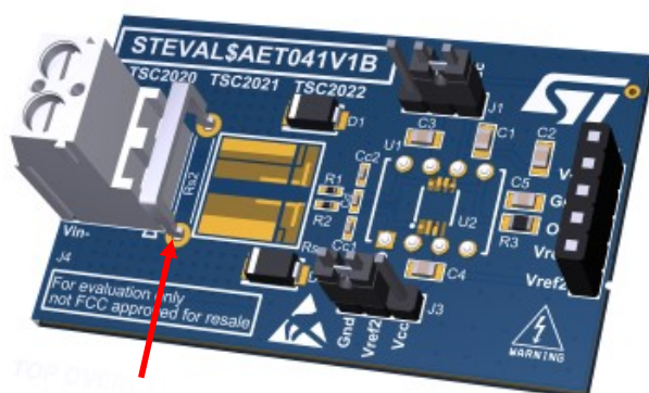
Figure 7. Shunt 2 wires connections
