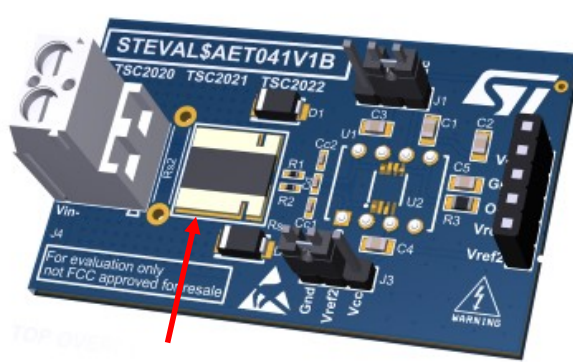
Figure 8. Shunt 4 wires connections
