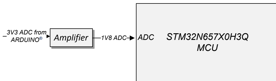
Figure 14. ADC/ARDUINO® input voltage adaptation
