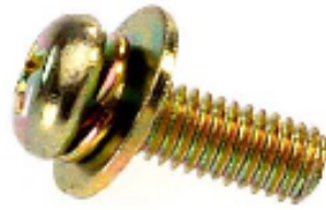
Figure 50. SEMS screw (size M3, spring washer 5.0 \Phi , plain washer 7.5 \Phi )
