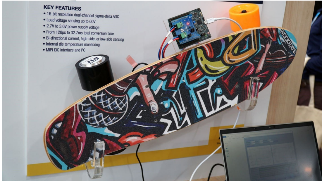
Figure 9. Skateboard demo using the TSC1641 and the STM32H5 to communicate in I3C
