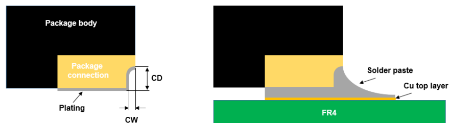
Figure 38. Wettable flank profile
