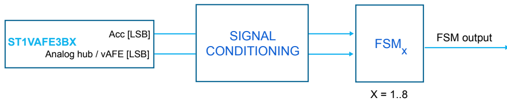
Figure 16. State machine in the ST1VAFE3BX
