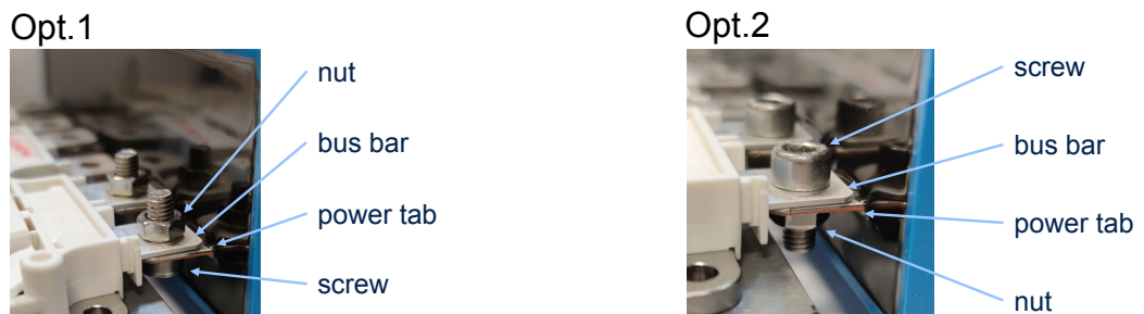
Figure 16. Example of power tab connections
