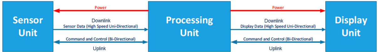
Figure 2. Data and power structure
