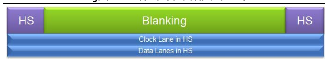
Figure 142. Clock lane and data lane in HS
